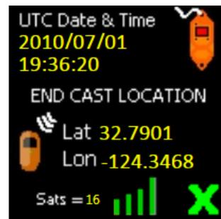
When complete, the CastAway™-CTD automatically loads the cast into the review data screen to allow immediate review of data quality ([Section 4](#)).
