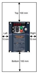
Figure 2.1 Mounting Direction and Required Clearances
