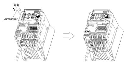
Figure 2.6 DC Reactor Connection
