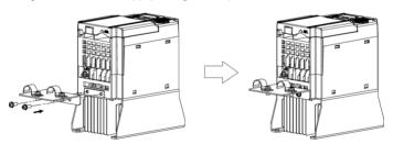
Figure 11.1 Attaching the EMC Grounding Flange
