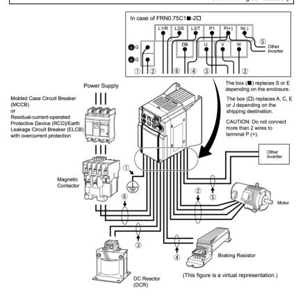
Figure 2.3 Wiring Procedure for Peripheral Equipment
