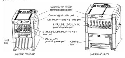
(\* When connecting the RS485 communications cable, remove the control circuit terminal block cover and cut off the barrier provided in it using nippers.) Note: A box (□) in the above model names replaces A, C, E, or J depending on the shipping destination.
