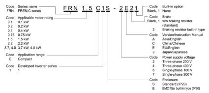
**Note:** When "None" and "w/o braking resistor (standard)" are selected in the built-in option and brake in the above codes, respectively, the type of inverter is written without the last 2 digits as a standard model.
