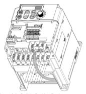
Figure 2.9 Built-in Braking Resistor Connection
