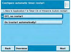
► Specify whether or not there should be an automatic restart after the timer-controlled function has been triggered.
