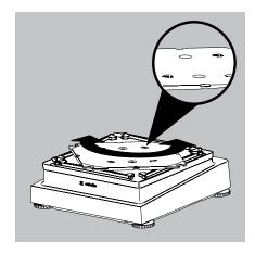
Carefully turn the pan support clockwise until the two buttons engage. The pan support is now attached.
