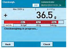
If the results are outside of the tolerance, the weight results are displayed in red (above maximum) or yellow (below minimum) on the graphic scale.
