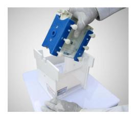
With the cam pin handles facing directly downwards, turn the cam pins fully through 180 degree or until th insert has tightened into the silicone mat. It is best to turn the cams in opposite direction to each other. Do not over turn as this will cause the glass plate to push upwards and the assembly will be more likely to leak.
