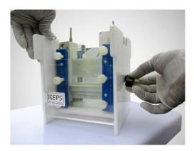
**Note:**Always reverse the silicone mat after casting avoid indentation from persisting. Never leave the casting up-stand with glass plate tightened into the outer tank for long periods of time while casting as this will also cause identations in the silicone mat.
