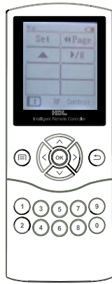
Fig. 13 RF panel interface
