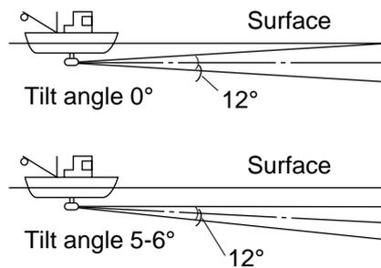
*Figure 2-2 Tilt angle and sea surface reflections*
