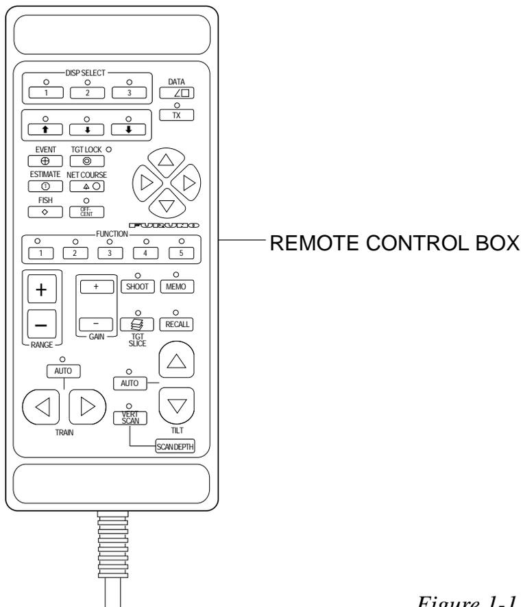
Figure 1-1 Display unit and remote control box
