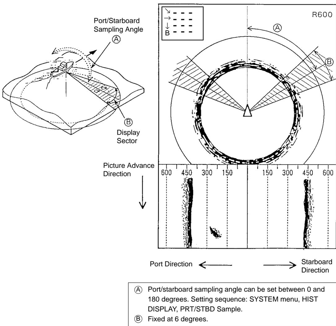
Figure 8-1 Port/starboard display
