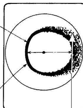
The deeper seabed echo is displayed in a weak color and with a long tail.
