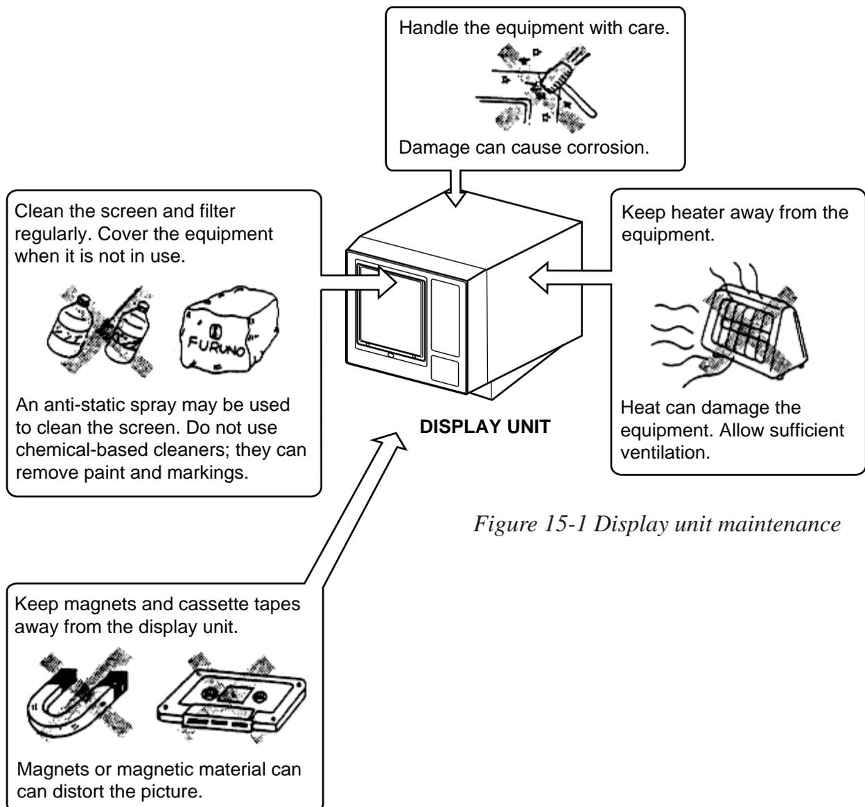
*Figure 15-1 Display unit maintenance*
