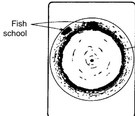
When the tilt angle is shallow, the reflection echo from seabed is weak and the fish echo which appears from bottom is easy to find.
