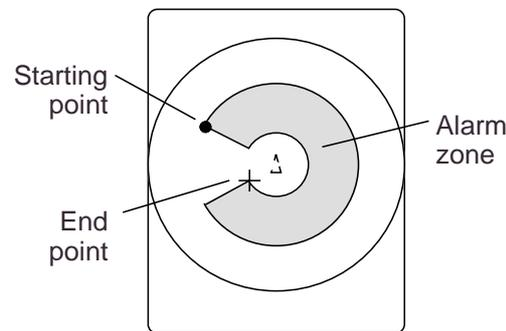
Figure 7-6 How to set the fish alarm zone
