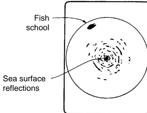
Seabed echo not displayed because of narrow tilt angle. Sea surface reflections are present.
