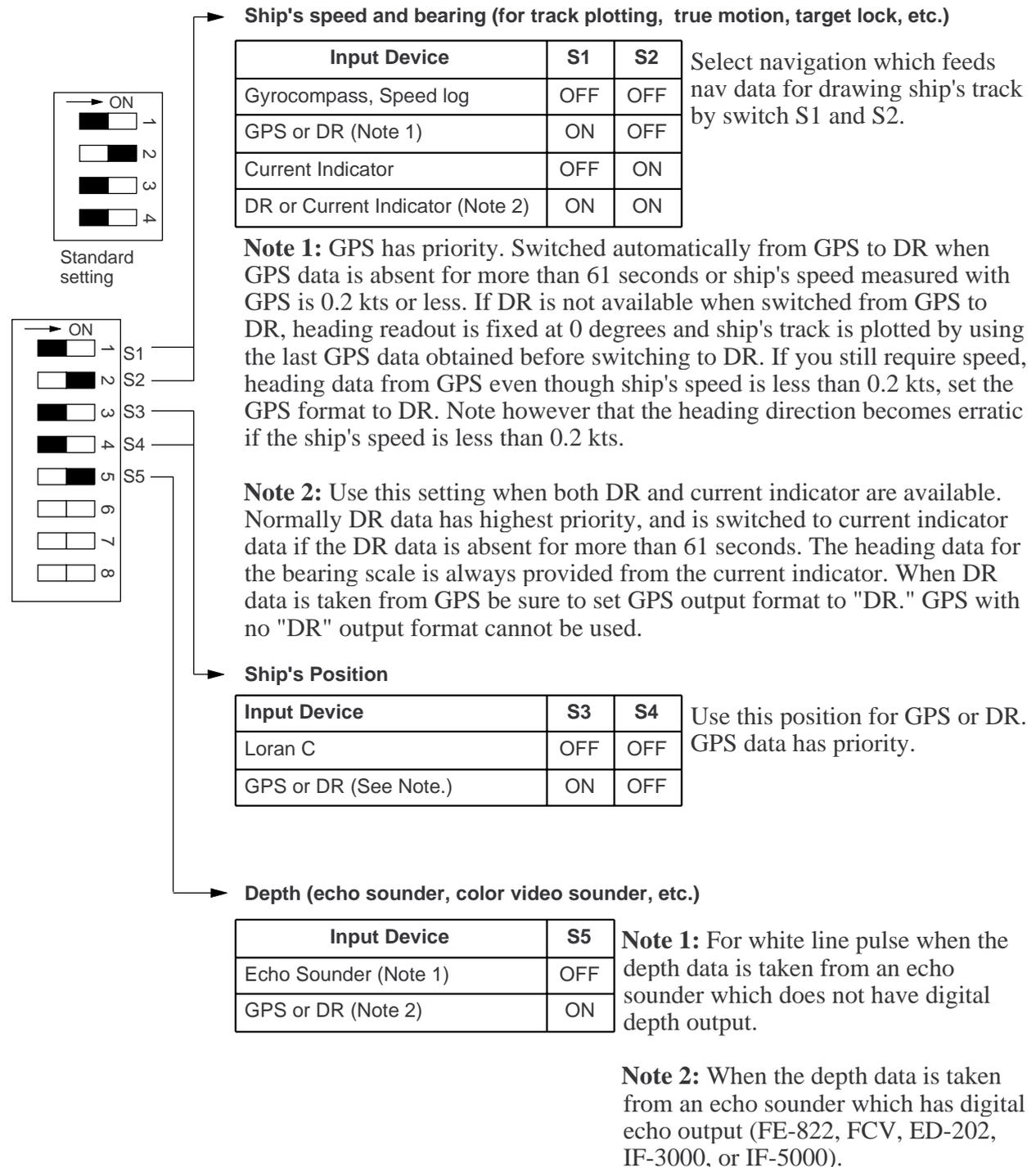
Figure 14-1 DIP switch settings in the interface unit
