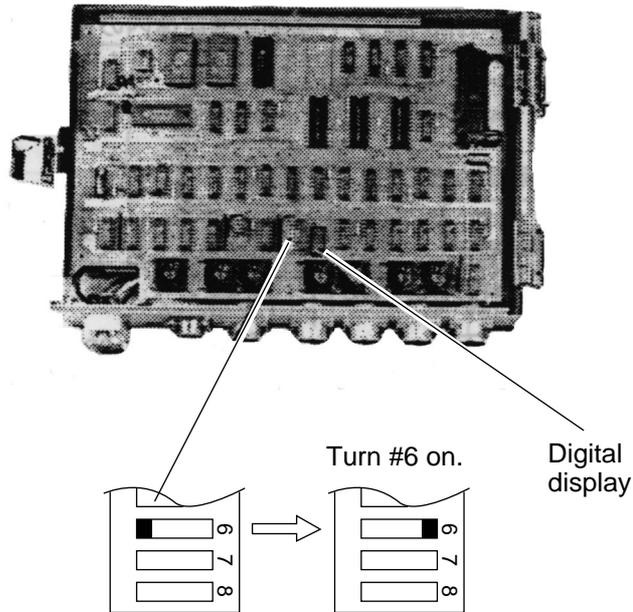
If the readout shows "0" the unit is functioning properly. If it is not working properly any of the following nine numerals or six alphabets appear.
