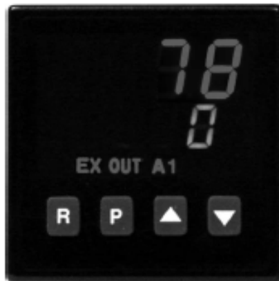
Figure 12: Typical Redundant Safety Controller Display
