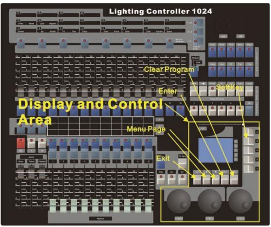
The Menu softkeys (labelled A – E) are used to select control options. The display next to the buttons shows what each one will do. The options for each key change depending on what the console is doing.
