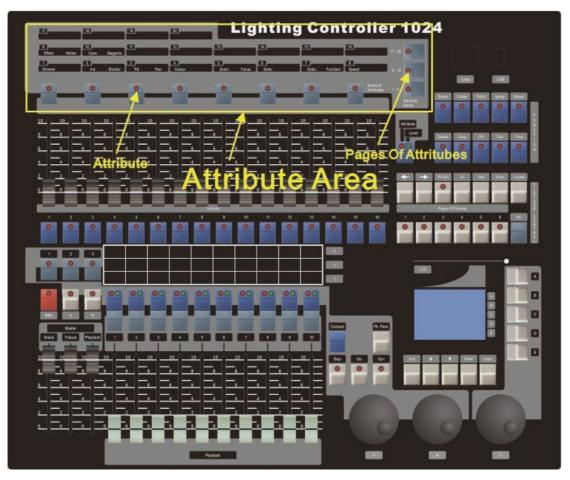
The Attribute buttons are used to select which attributes of a fixture (e.g. colour, gobo, pan, focus) are going to be controlled using the Control wheels. The buttons have lights on to show you which attributes are active. The bottom (red) button allows you to reduce the intensity of a fixture if it loses position during a show.
