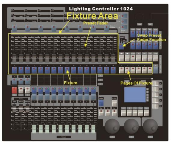
There are 6 pages of fixtures supporting up to 96 fixtures. The <Swap Preset Fader Function> button with 2 LED indicators can be used to switch the functions of the 16 faders. When <Attribute> is activated, the faders are used to adjust the value of attribute which above the faders; When <Level> is activated, the faders are to adjust the intensity of fixtures.
