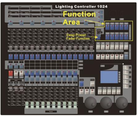
Fixture control area: including buttons of <Previous>, <Next>,<<HiLight>, <All>, <Odd>, <Even>, <Locate> and <ML>, which are functions to control the fixtures.
