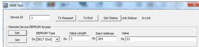
Step 6: Now for the ULE Controller Side. Close the HAN Test Window and return to the Main Window and Click on the EEPROM Read/Write button at upper right
