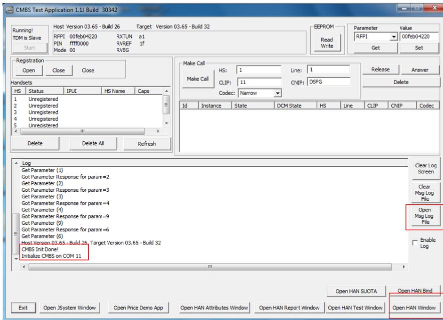
The log window shown above is an abbreviated version of the incoming/outgoing flow of information at the CMBS UART Interface. A more detailed (message) log is recorded in a file that can be opened from the button indicated above. This file is located in the same directory as the DSPG Test Application.exe file.
