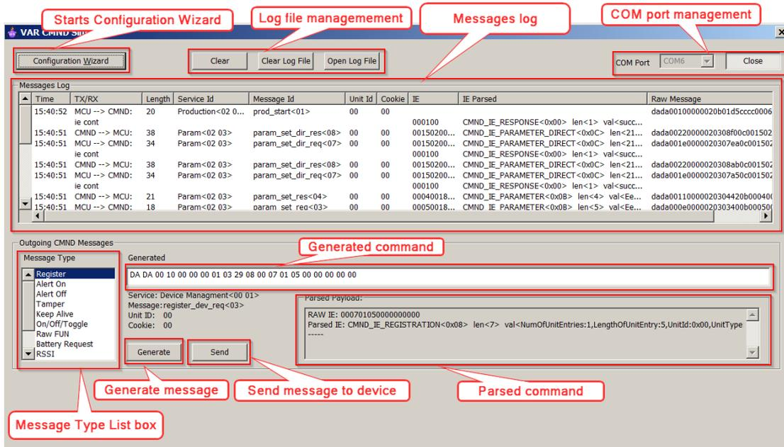
Go to the “Message Type” window, pull down “Get Version”, hit “Generate Message” button then “Send”. You should see the “req” and “resp” between the VAR (=MCU) and the DHAN (=CMND), as shown below.
