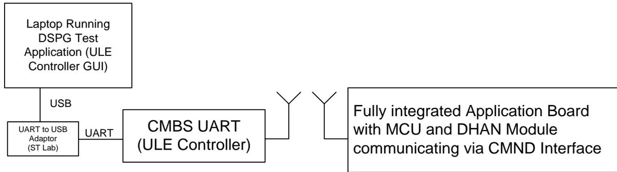
The User designs an application board which integrates a favorite MCU, sensors/switches, the DHAN module and a 2GHz antenna. Prior to designing this application board, the User should discuss application needs and constraints with DSP Group to insure that the application schematic is optimal as well as receiving the SW training and detailed documentation needed to create an full-fledged application.
