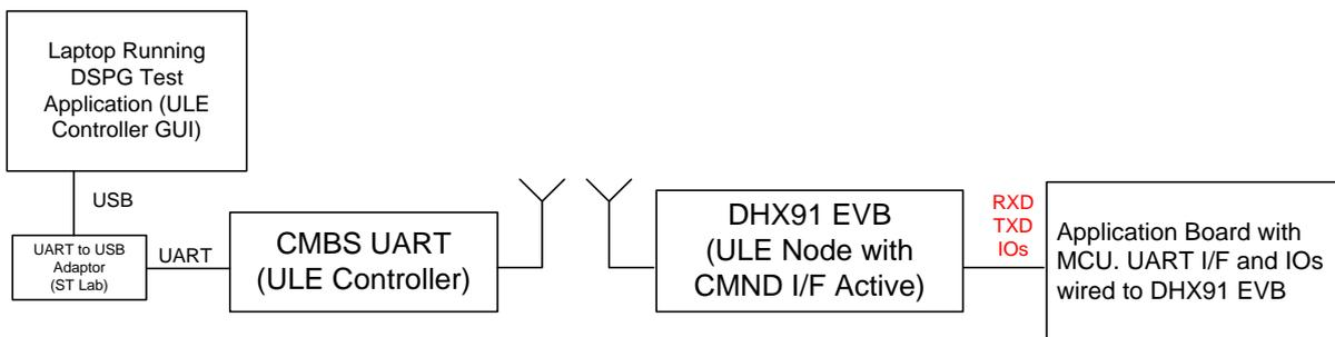
ULE transactions have been embedded into the Application SW and their effectiveness can now be validated. User will be able to register (=pair) his ULE Node Application with the ULE Controller, send maintenance (= Keep Alive) and simple Alarm/Event messages, turn actuators ON-OFF, send battery and RSSI status over to the Controller.
