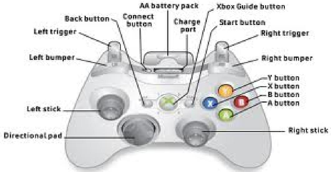
Figure 2.11 XBox 360 Controller Layout
