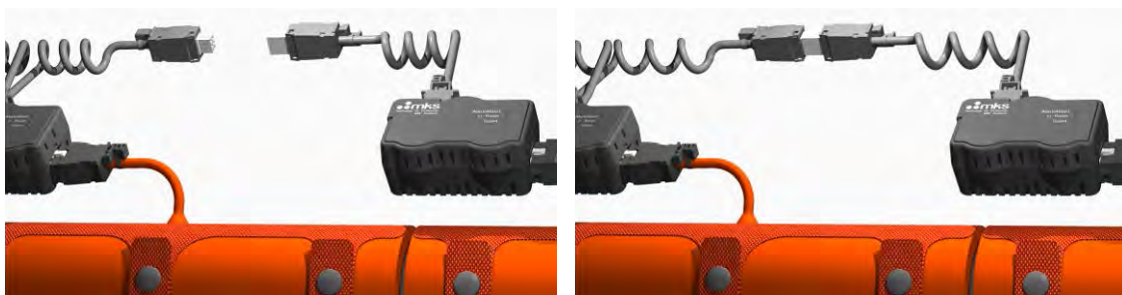
Connecting power cables
