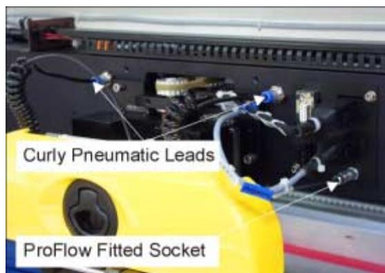
5. Connect the pneumatics and switch the machine to **ON**. To ensure that the machine recognizes the ProFlow module, the following indications on the machine MMI are evident:
