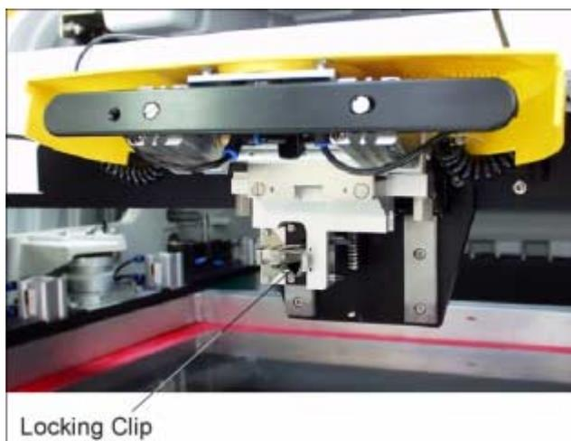
3. Locate and fit the ProFlow transfer head unit to the pressure mechanism by means of the two locating dowels. Slide the unit onto the pressure mechanism. Once the unit is slid fully home, it is secured by closing the locking clip.
