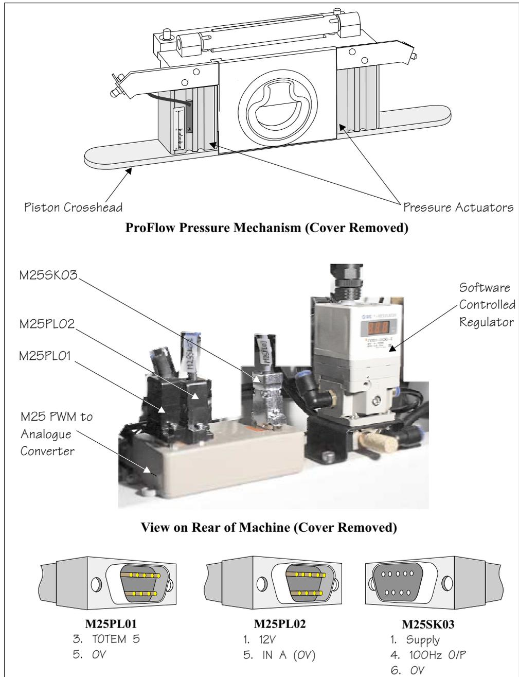
**Figure 9-16 Software Controlled Pressure Mechanism**
