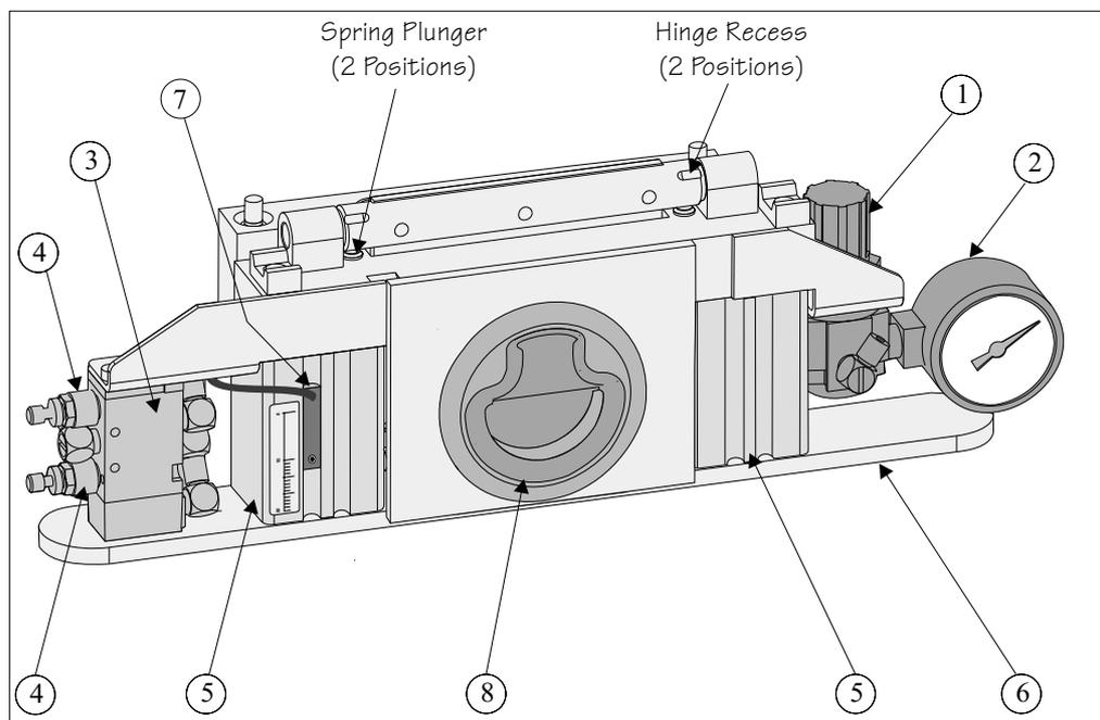
**Figure 9-4 Pressure Mechanism Elements (cover removed)**
