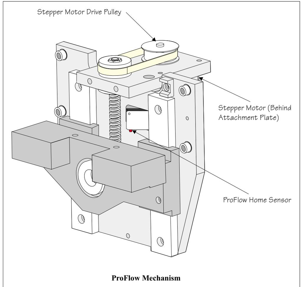
**Figure 9-17 ProFlow Mechanism Motor and Sensor Location**
