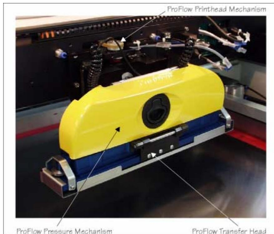
**Figure 9-1 ProFlow Fitted to the Machine**
