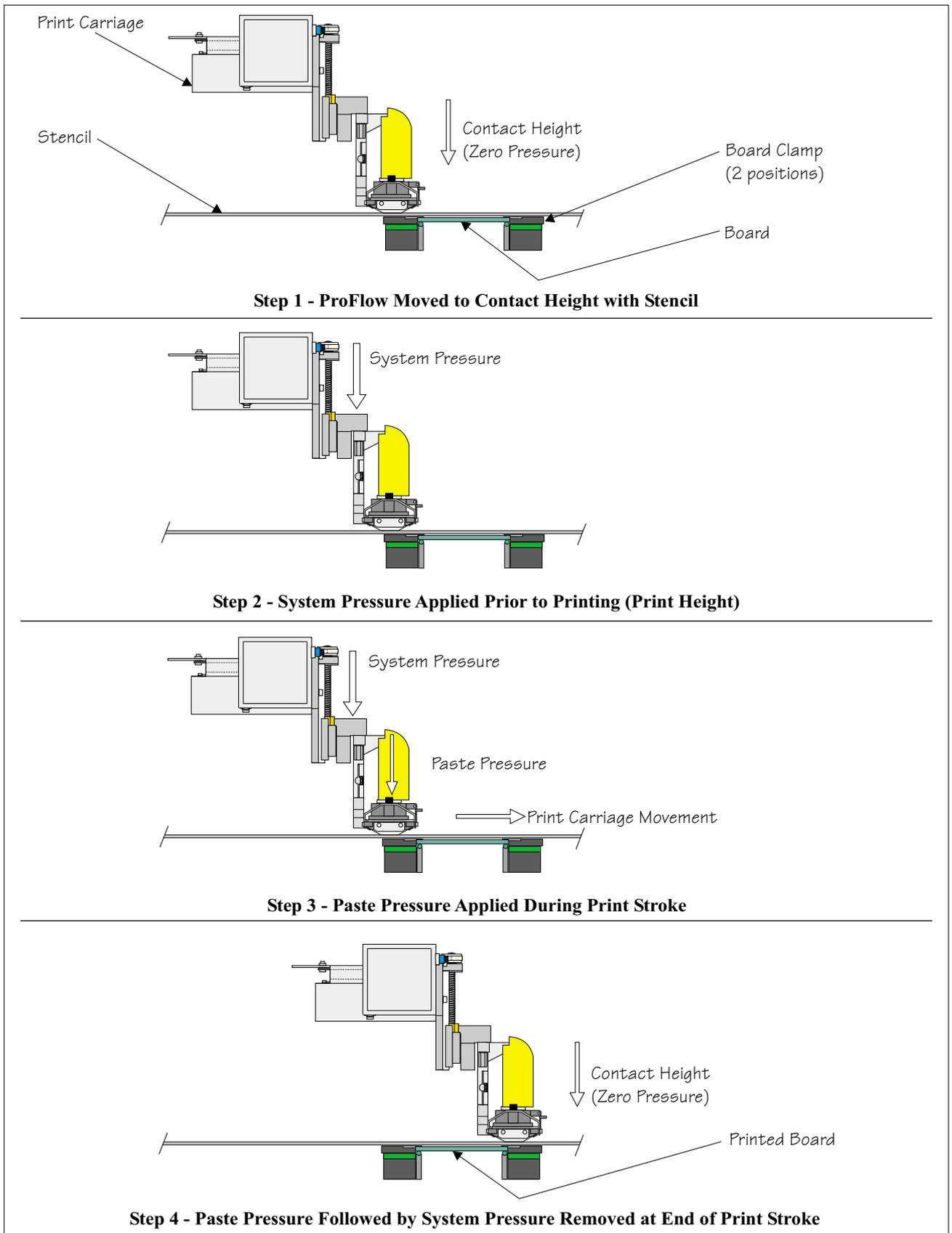
**Figure 9-20 Side View of ProFlow During Print Cycle**
