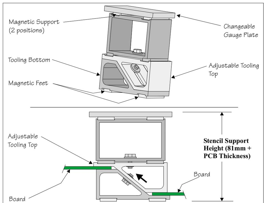
**Figure 9-26 Setting Up Stencil Support Height**
