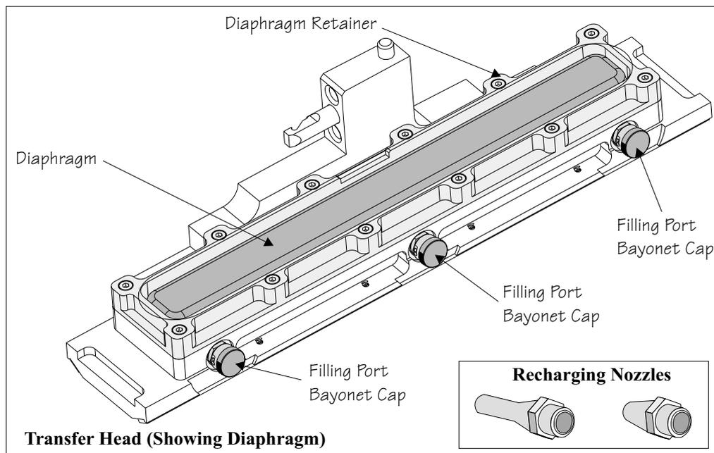
**Figure 9-12 Rechargeable Transfer Head**
