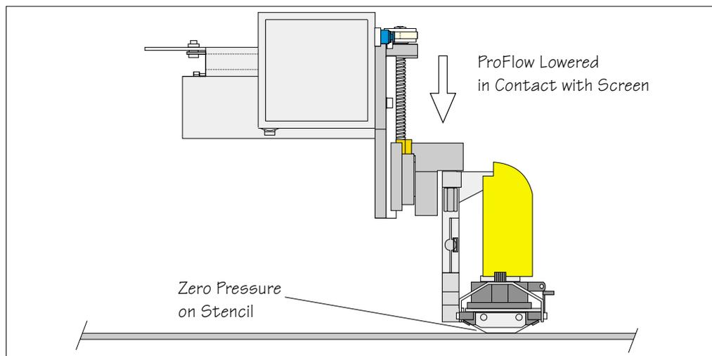
**Figure 9-22 ProFlow in the Contact Height Position**
