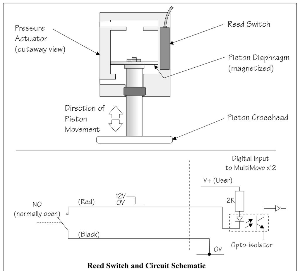
**Figure 9-19 Reed Switch and Circuit Schematic**
