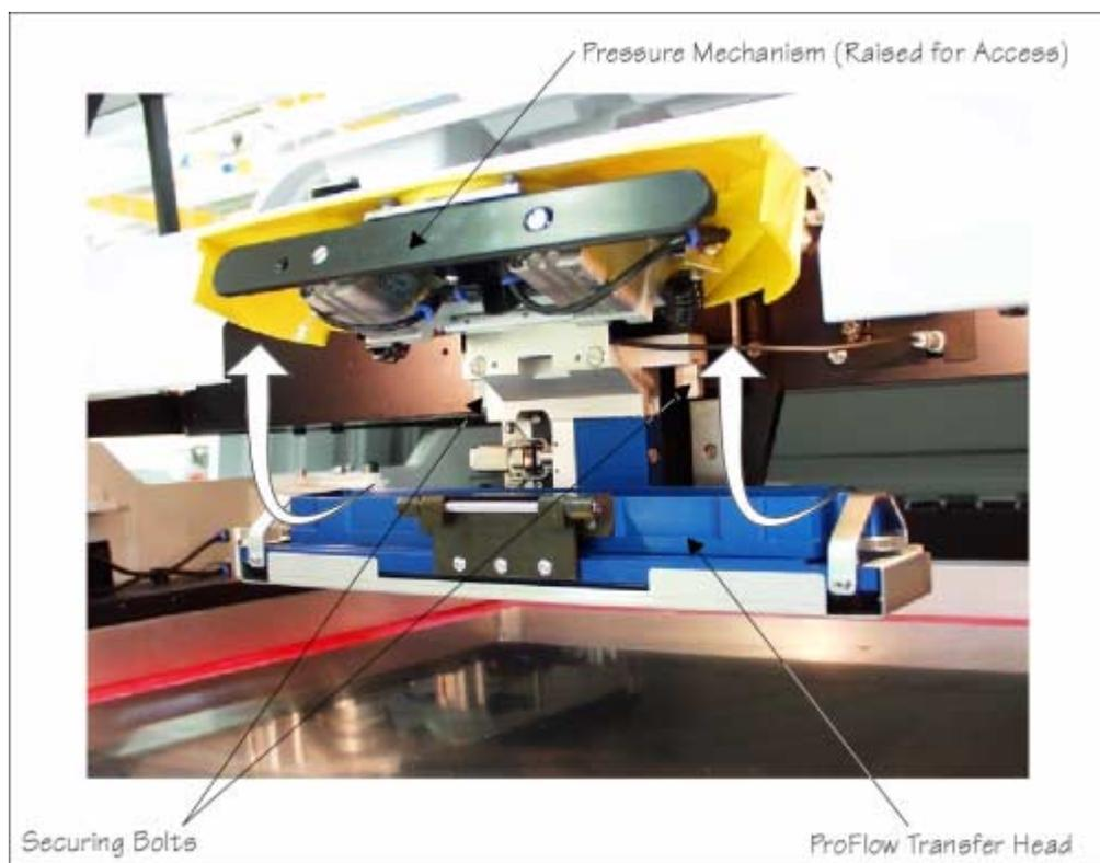
**Figure 9-5 Pressure Mechanism Raised for Access**
