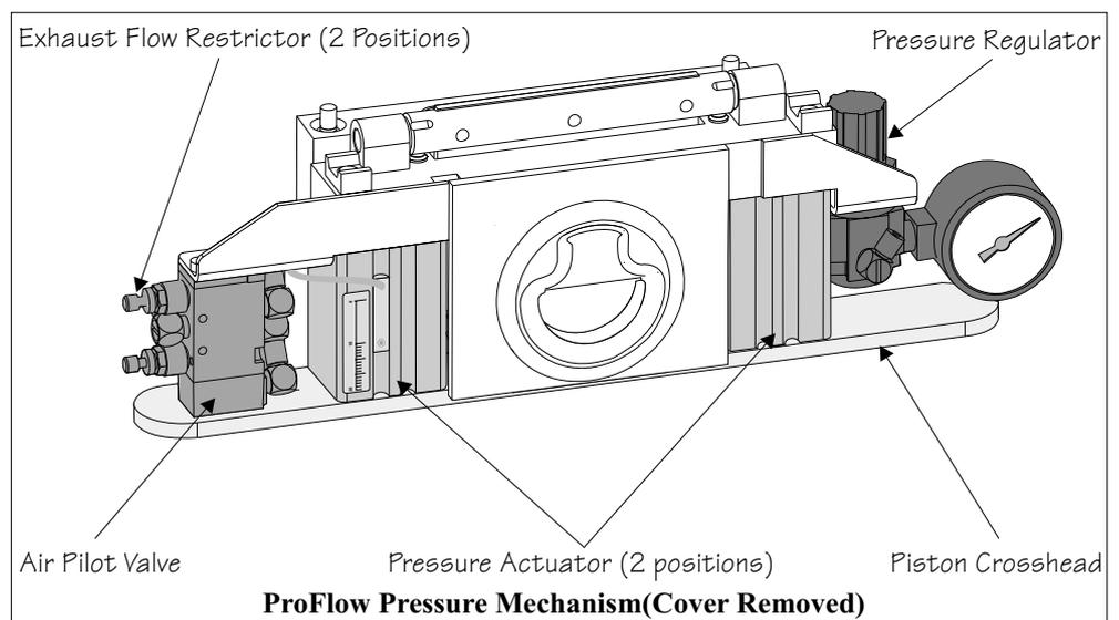
**Figure 9-15 Pneumatic Supply Main Components**
