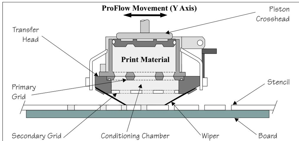
The dual conditioning chamber, was partly developed from knowledge gained with the single conditioning chamber. This to ensures maximum print material transfer and optimization on more demanding process platforms, the print material is driven around the two individual side chambers, in the same manner as above.
