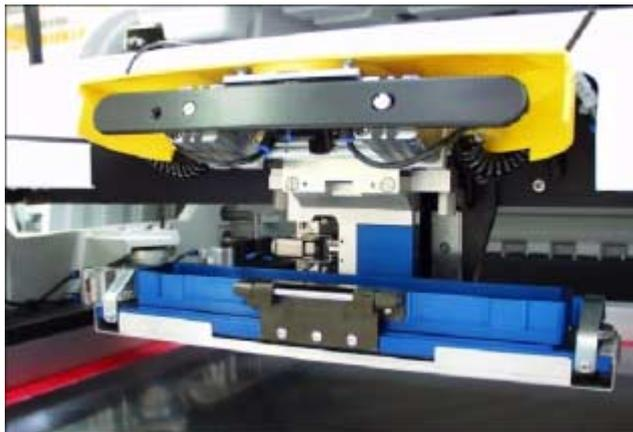
4. Lift the light shroud for access and plug the electrical connection ProFlow Fitted from the ProFlow unit into the socket sited on the right hand side of the ProFlow on the print carriage, (figure below refers).
