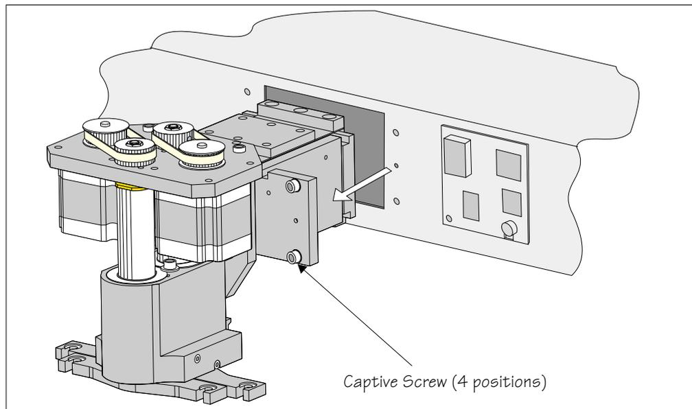
6. Position the ProFlow printhead mechanism locating dowels into the print carriage and secure the unit by means of the four captive screws, using a **4mm** Allen key (see figure below).
