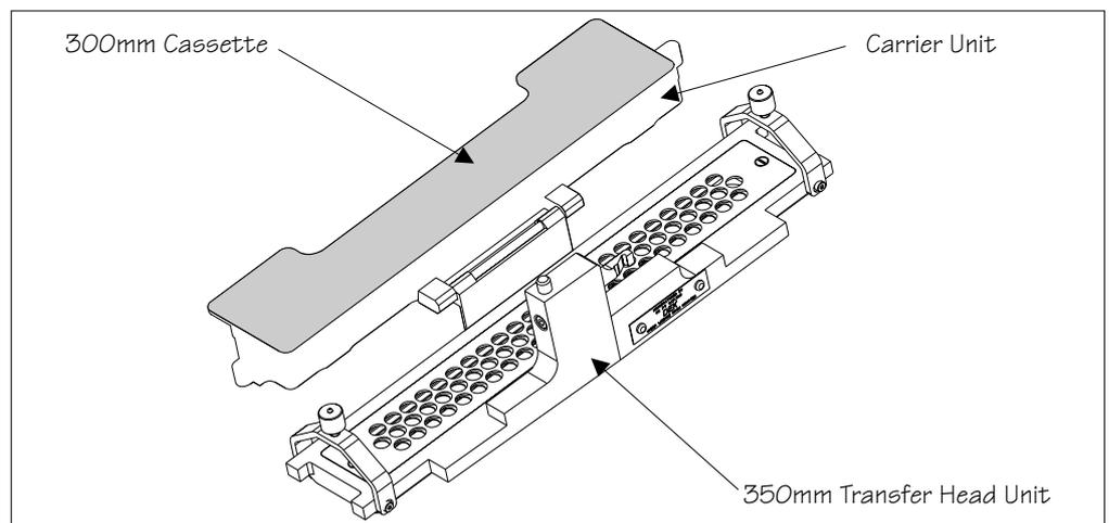
**Figure 9-8 Transfer head (350mm)**
