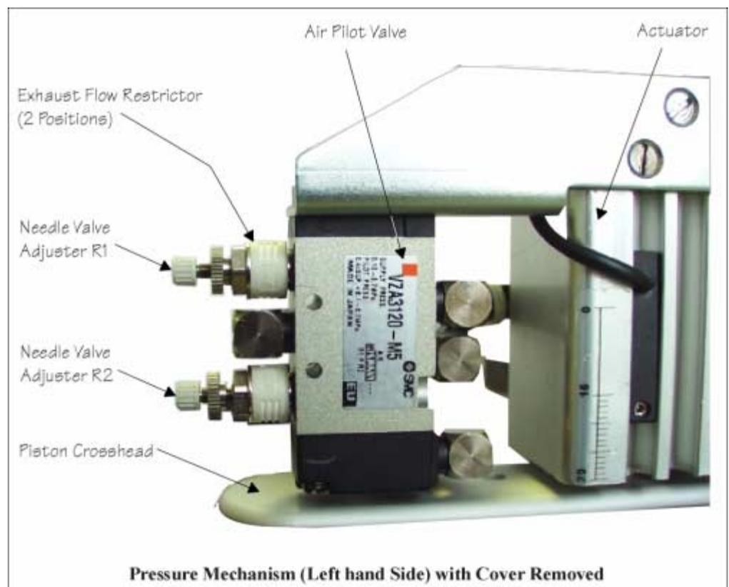
**Figure 9-25 Exhaust Flow Restrictors**
