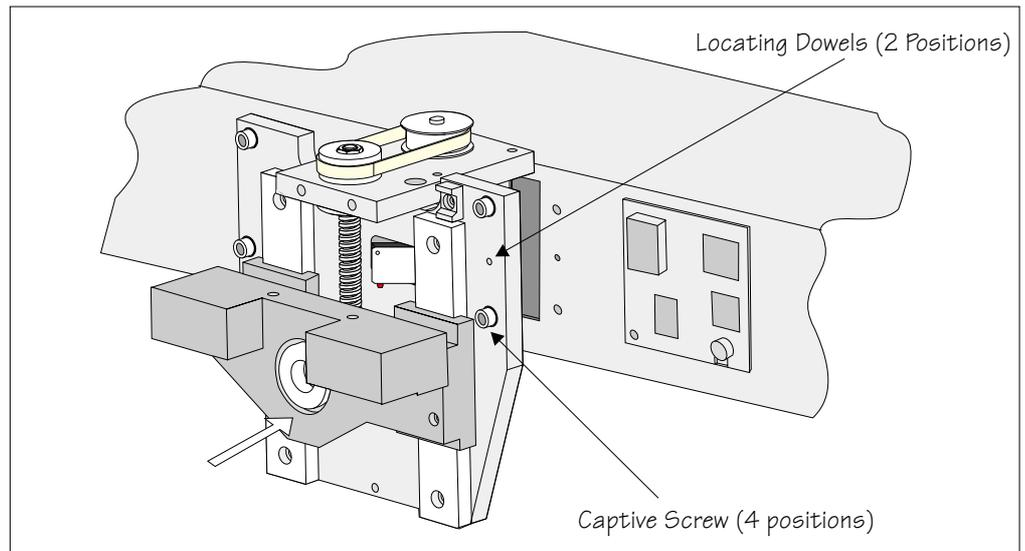
7. Fit the following ProFlow mechanism connectors (figure below refers):
