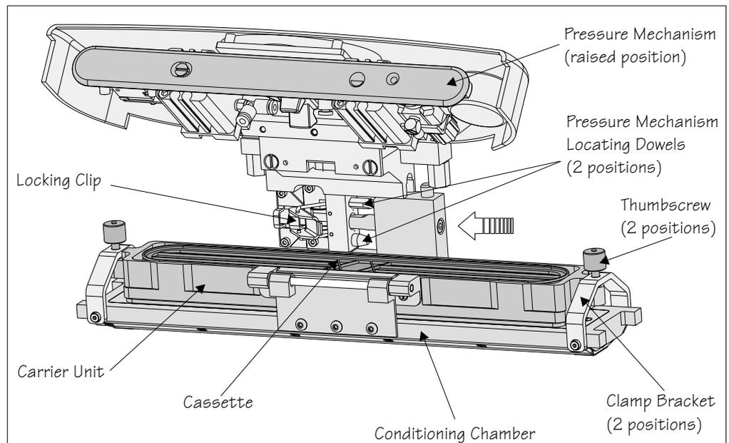
**Figure 9-7 Transfer Head to Pressure Mechanism Interface**
