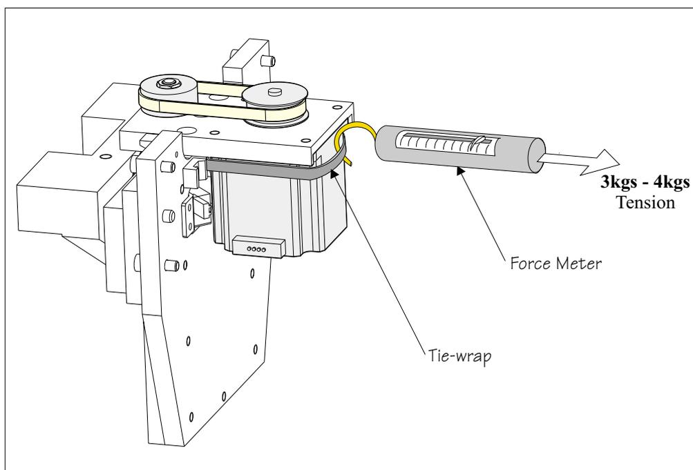
8. Pull the force meter until a tension of **3-4kgs** is monitored on the meter. Tighten the four screws whilst the motor is under tension.
