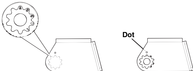
Align plastic ratchets in bracket.
