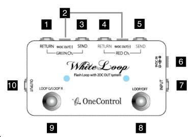
Effects connected to Loop Red and Loop Green, while being powered, can be bypassed with a true bypass switch. Effect 1 and 2 can be turned off with the Red and Green switch with one action.
