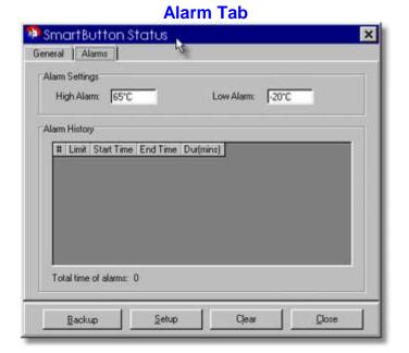
The Alarm Tab displays the high and low temperature thresholds. Once the temperature exceeds this range, the SmartButton automatically starts to record data.
