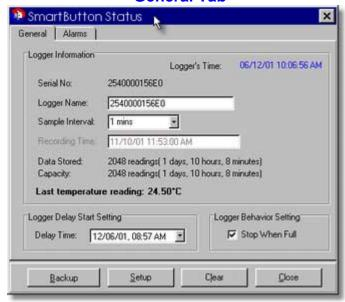
The General Tab displays an overview of the SmartButton's operational parameters.
