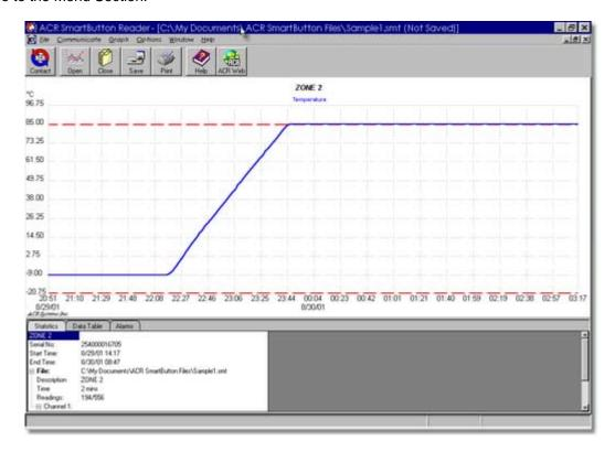
Referring to the above picture, you will find at the top of the window the **menu bar** containing items used to control the application; File, Communicate, Graph, Options, Window and Help. These are the basic menu headings, where you will be able to locate individual functions within the software. To learn more about the role of each sub menu feature, please refer to the various **Menu Options**.
