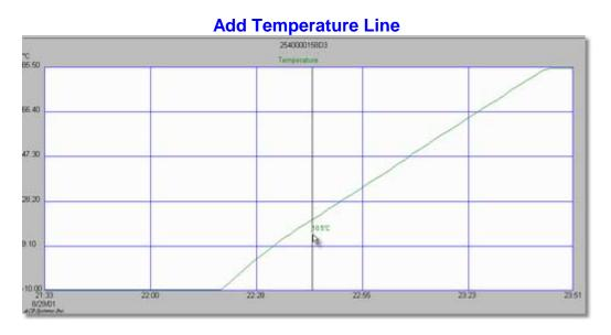
To erase the temperature line on a graph, move the mouse pointer to the line and click the Left mouse button on the line. Release the mouse button and the graph displays a box at the center of the temperature line. Once the box is visible, press the Delete button on your computer:
