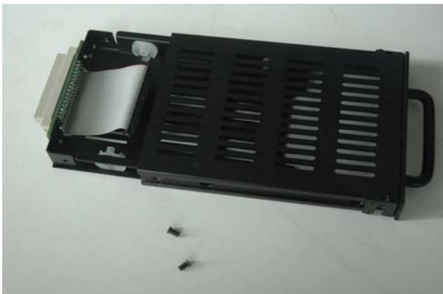
Process 3: Connect HDD, take care the direction of HDD connection, don't install in wrong direction
