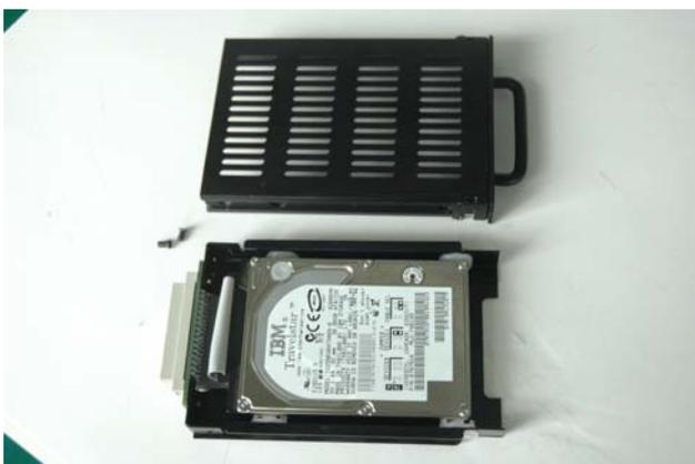
Process 4: Put the HDD through the rubber shock proof mat, and fix the HDD on the mat
