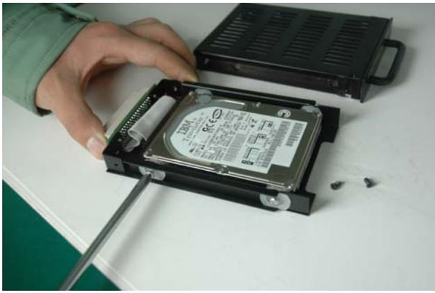
Process 5: Seal the HDD by upper cover after fix up HDD
