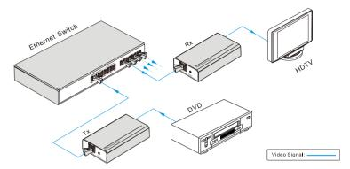
One or more receiver may be utilized in this case to broadcast signal from 1 transmitter to 1 or more receiver.
