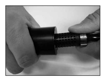
1. Insert the diffuser into the socket.
