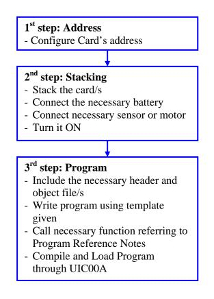
A basic setup for IFC-CP04 will be illustrated this chapter. Please ensure the power is **OFF** before inserting or removing IFC card.
