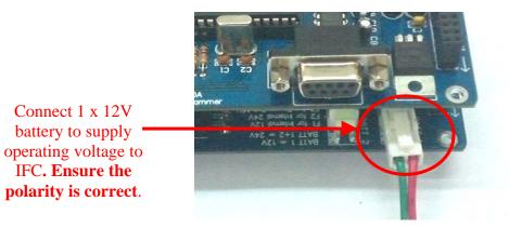
d. Turn ON the IFC power by pushing the toggle switch to "ON". There should be at least 3 LED (12V LED on Power Card, PWR LED on Main Brain and PWR LED on Control Panel) light up as shown.
