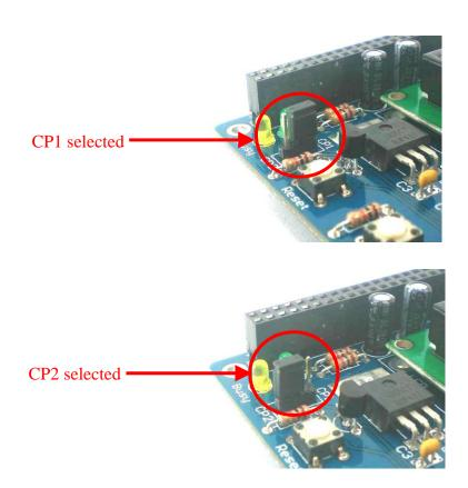
Please switch ON the power on Power Card, the PWR LED of IFC-CP04 will turn ON as shown in figure below. Initially, if there are no functions related to IFC-CP04 being called in Main Board's program, the screen of LCD will not show anything and the LCD backlight will not turn ON.
