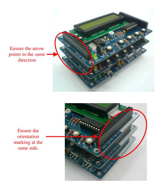
**Cautions:** Please ensure that every card is being stacked properly in correct orientation. Whole IFC system will be damaged if one of the cards is being stacked wrongly when it is powered up.
