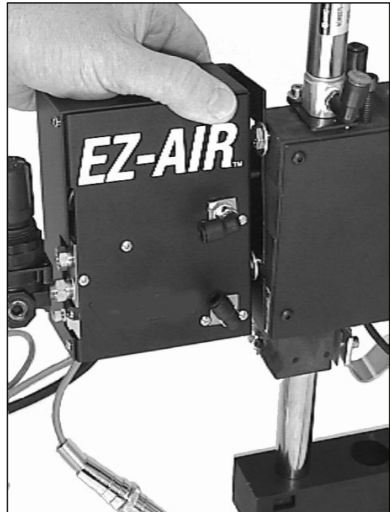
Figure 2-2. Installing EZ-Air On Model 80A or 86A Weld Head
