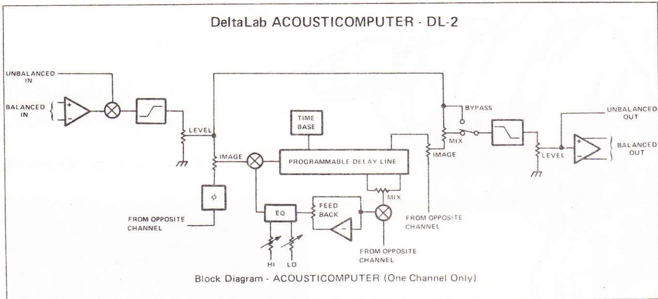
**Fig. 1: DeltaLab DL-2: Block diagram of the unit (one channel only).**
