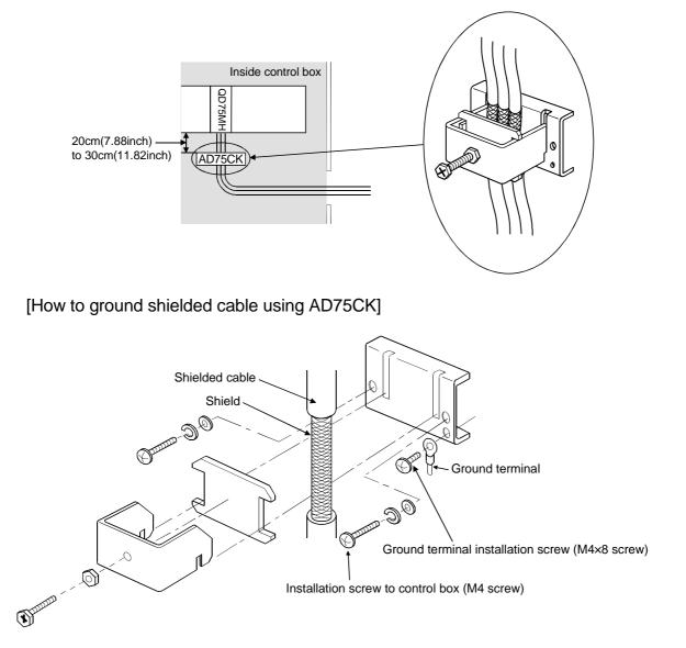
Using the AD75CK, you can tie four cables of about 7mm outside diameter together for grounding.
