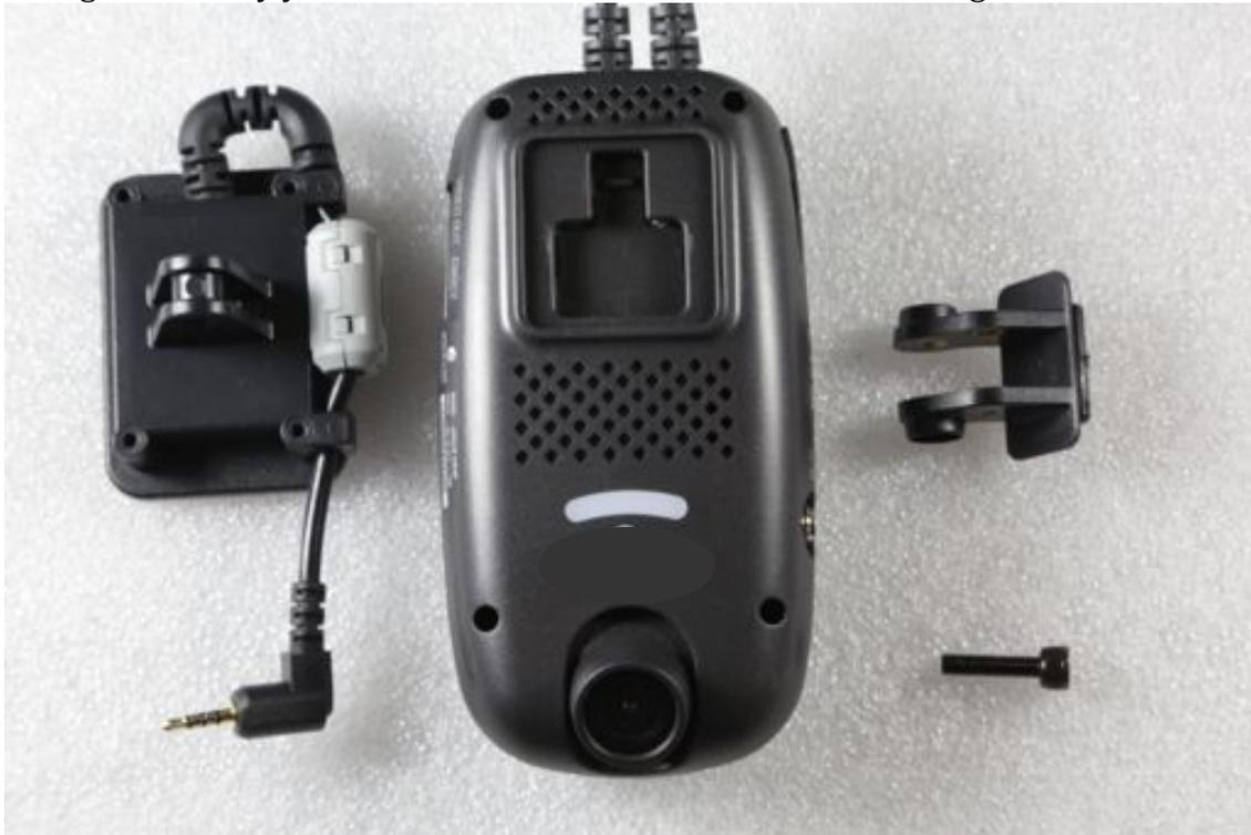
1. Attach the mount head to the GPS Bracket as seen in the image below
