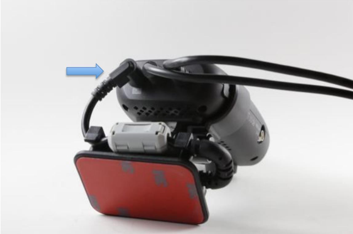
7. (Optional) With the camera facing you, attach the Wi-Fi antenna to the port located on the left hand side of the camera.
