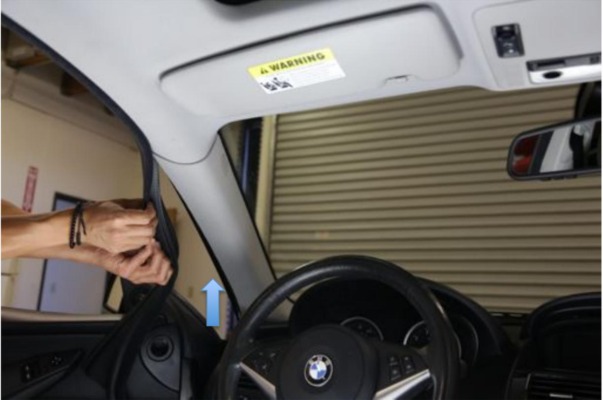
13. Place the male jack from the wiring harness close to the female jack from the camera allowing for a bit of slack and begin to tuck the wiring harness cable towards the fuse box going through the top of the support pillar. Once the end of the harness with the power and ground wires reaches the fuse box, reapply the door seal concealing the cable.
