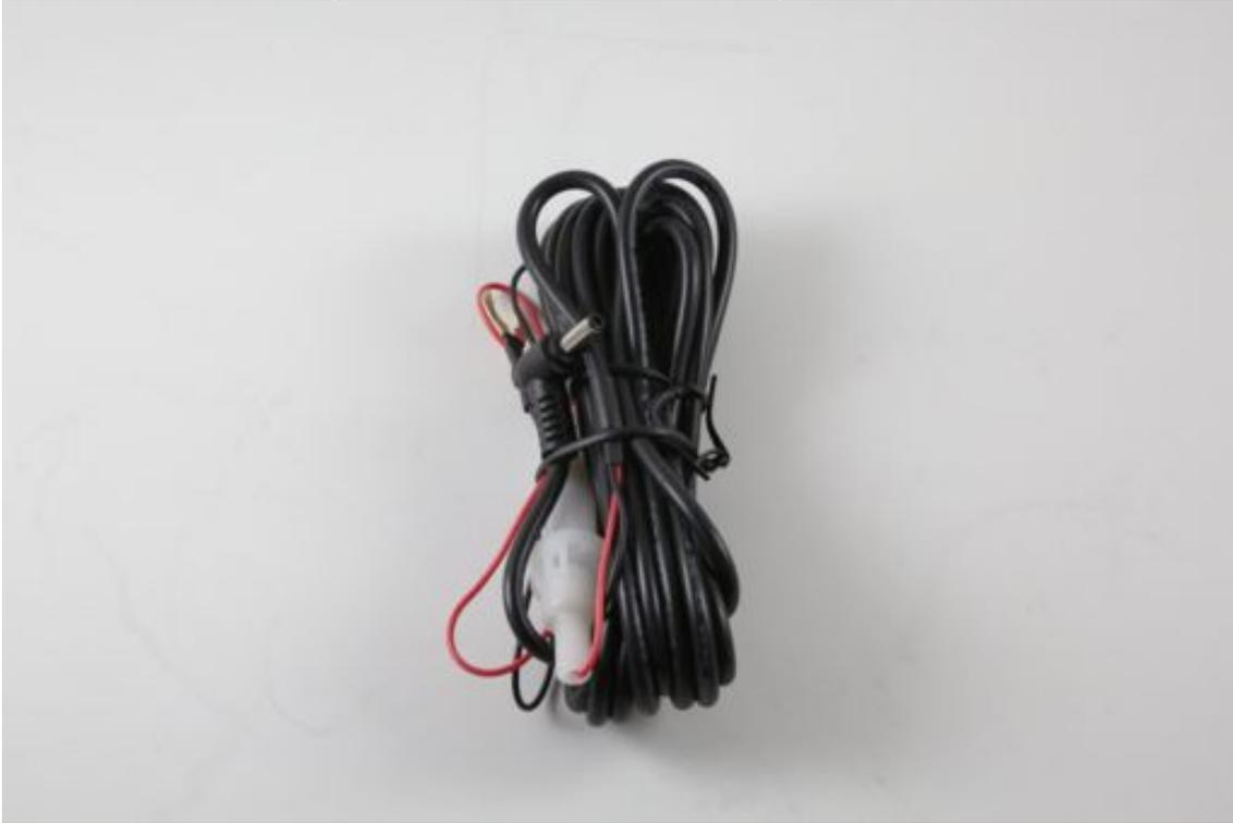
12. On one end you have the power wire (A. red wire) and the ground clip (B. black with gold clip attached). On the opposite end you have the male jack connector (C.). Strip  $\frac{1}{4}$  of an inch of the protective sleeve off of the power wire (A. redwire)
