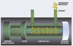
Filtered infrared energy is absorbed by the refrigerant present in the sampling cell, causing D-TEK Select to alarm.
