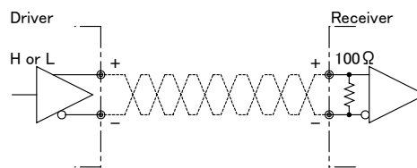
Figure 3-3-2 Circuit of LVDS
