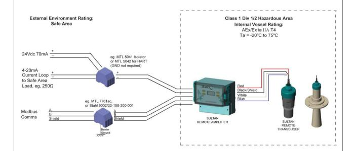
Note 1. Wiring to conform to NFPA-70
