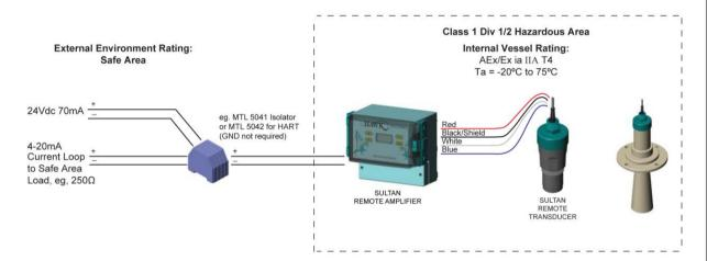
Note 1. Wiring to conform to NFPA-70
