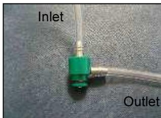
1) Connect pipe work to flow adaptor
