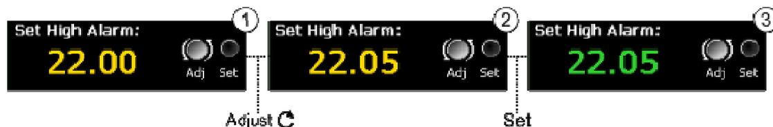
**Figure 31 - Example of alarm set-point adjustment**
