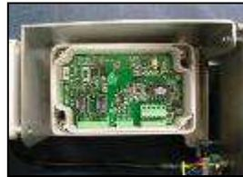
4) Tighten the M4 Pozi Pan screws
