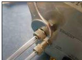
4) Secure pipe work in place with securing nuts
