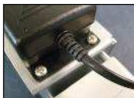
2) Secure in place with the supplied M4 x 8mm Pozi Pan screws
