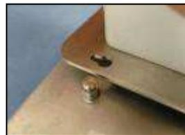
8) Align mounting hole with standoff
