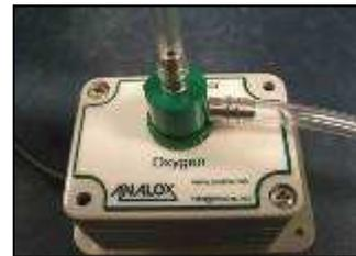
The MEC sensor sample input line can also be piped to a dedicated SDA flow adaptor unit or connected to the exhaust of the SDA CO<sub>2</sub> sensor module.
