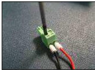
4) Secure using a terminal driver
