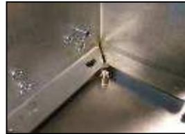
2) Align mounting hole with standoff
