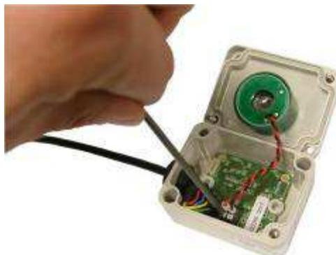
Figure 47 - Disconnecting the cell
