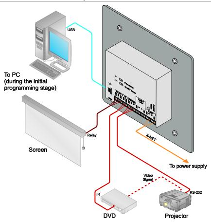
Figure 8: Example of a Typical RC-63DL Configuration
