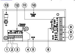
Figure 4: RC-63A Room Controller Rear Panel (for Europe)
