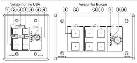
Figure 5: RC-63D Room Controller Front Panel
