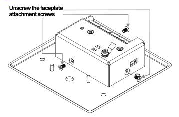
Figure 12: Unscrewing the Faceplate Attachment Screws
