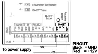
Figure 7: RC-63D Standalone Power Supply Pinout
