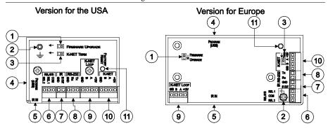
Figure 2: RC-62 Room Controller Rear Panel
