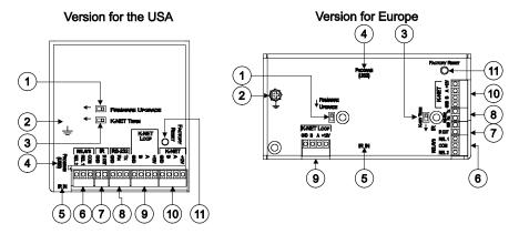
Figure 6: RC-63D Room Controller Rear Panel
