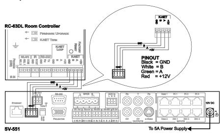
Figure 9: RC-63D connected to the SV-551 SummitView<sup>TM</sup> Processor / Switcher
