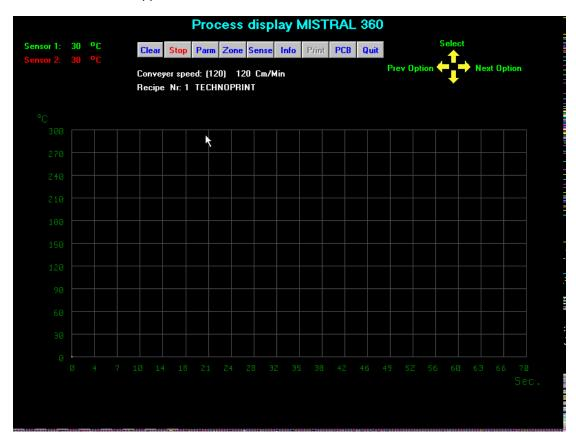
Note that there are now, sensors displayed on the top left of the screen. (depending on the type of Mistral oven connected) Also the diagram has been changed. The temperature axis is the same only the time axis is now different. This axis shows you the time that is needed for a PCB to pass through the oven. It is calculated from the conveyer speed and the length of the oven chamber. In this case it means that it will take 70 seconds for a PCB to pass all the zones in the oven.
