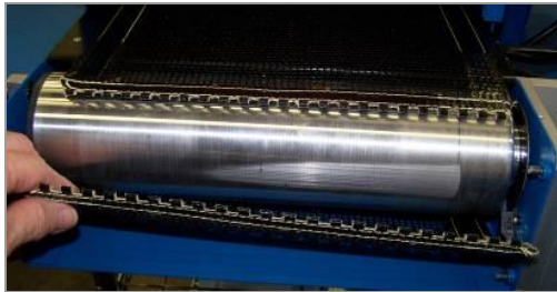
Figure 37. Run New Belt Around Conveyor Frame
