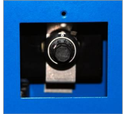
Figure 25. Blower Speed Control (Close Up)
