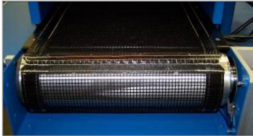
Figure 35. Place Splice at the End of the Conveyor
