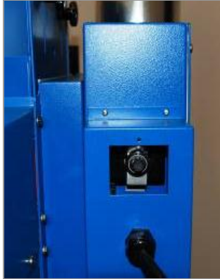
Figure 24. Blower Speed Control
