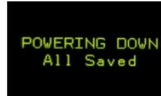
If the CR-1 does not shut down in 3 seconds, hold-in (about 6 seconds) to force shut down.
