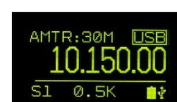
5. **Frequency Stepping [SCAN]** The CR-1 Steps sequentially through frequencies and does not stop on a channel or frequency if a signal is present.
