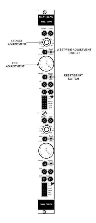
Fig. 2.1: Model V993 B front panel
