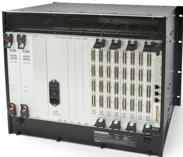
Figure 8-8. The TANDBERG MPS 800 V.35 interface cards
