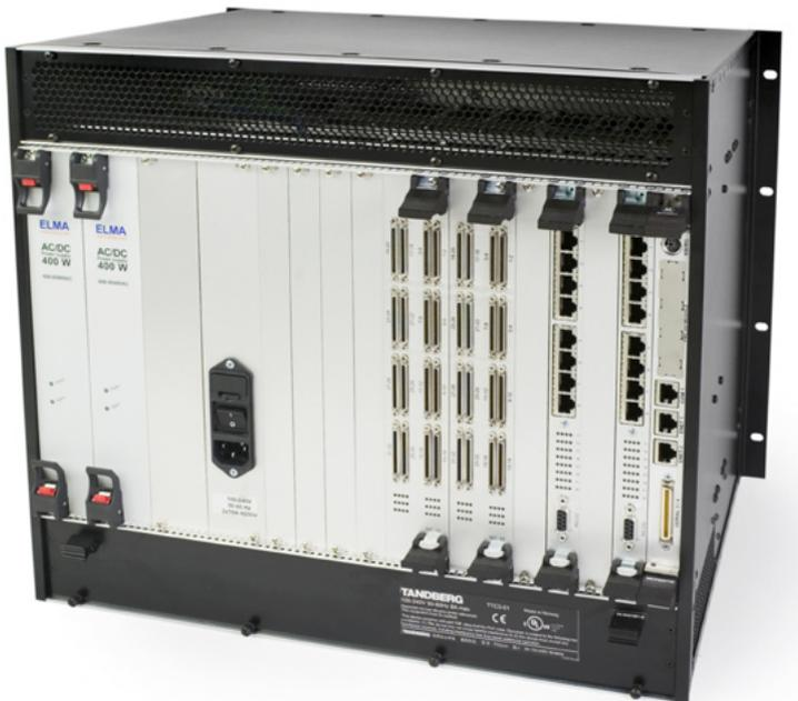
Figure 8-12. PRI E1/T1 and V.35 interface cards, MPS 800
