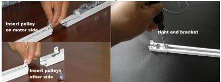
**Please note:** make sure that drive string is along inside wall of track and keep any carrier wheelers from interfering with the string.
