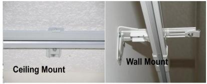
**Note**: All the brackets should be on the same surface in a straight line. Leave at least 5cm (2 inches) space between the wall and the track. The transmission box can be assembled on either the right or left side.
