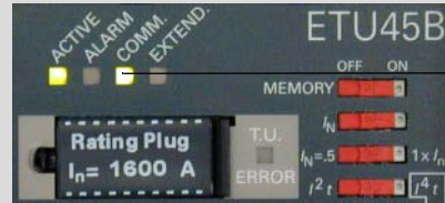
Fig. 2-1 Front view of the PROFIBUS module for the SENTRON WL with the PROFIBUS connection and the two LEDs. The figure below shows a section of the ETU45B and its LEDs for displaying statuses.
