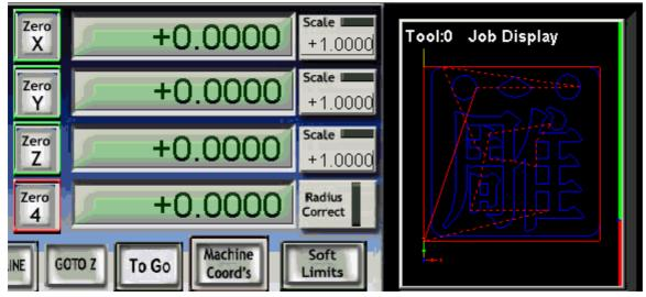
(3)Power on the control box driver, move the spindle tool bit to the left-bottom of the material board by manual control the three axis, the area in the red circle(the image below)is the safe area. The left bottom red-green WCS arrowhead above is the original point, move the spindle bit (without cutter) to this point.
