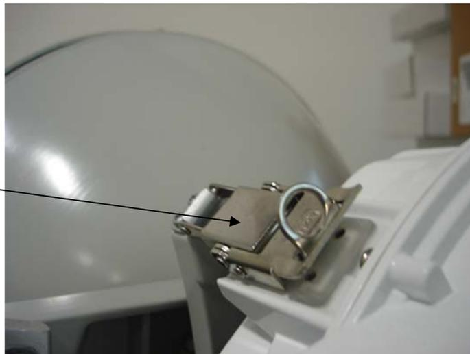
Figure 26 Mounting Latches
