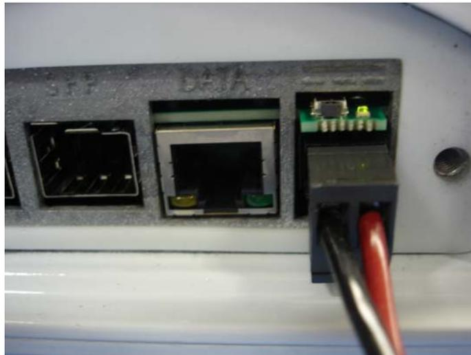
Figure 22 Direct Power Connector
