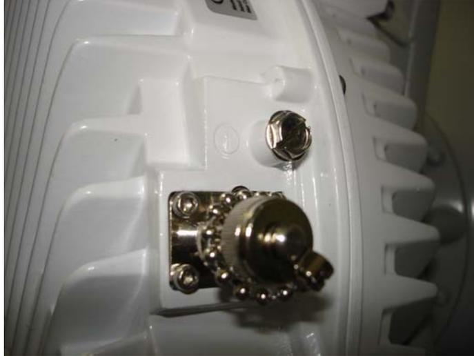
Figure 31 Ground Lug and RSSI BNC on StrataLink
