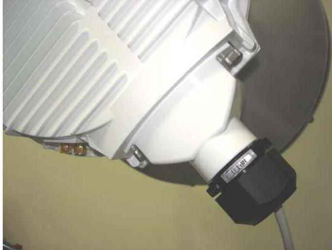
Figure 29 Port Cover/Cord Grip Installed
