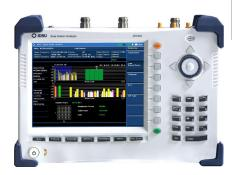
Spectrum Analyzer: 100 kHz to 4 GHz
