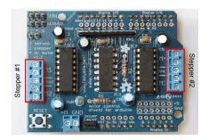
AF\_Stepper Stepper1(48, 1); // A 48-step-per-revolution motor on channels 1 & 2
