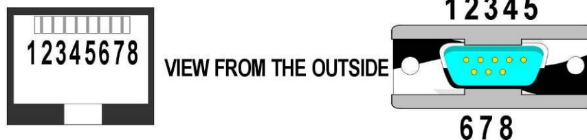
Making the RJ45 to RS422 male adapters
