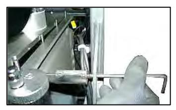
Figure 7-18: Unscrewing Lift Screw into Tab Hole (Step 14)
