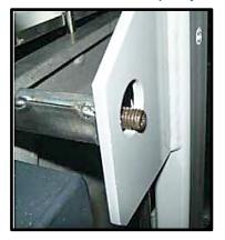
Figure 7-19: Lift Screws Extended into Tab Holes, Left and Right Sides (Step 14)
