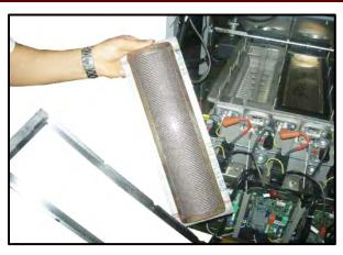
Figure 7-23: Removing Individual Burner Module and Gasket (Step 1)
