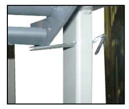
Figure 7-22: Lift Pins Inserted into Lift Holes, Left and Right Sides (Step 15)
