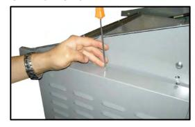
Figure 7-5: Remove Screws at Edges and Remove Side and Rear Panels (Step 3)
