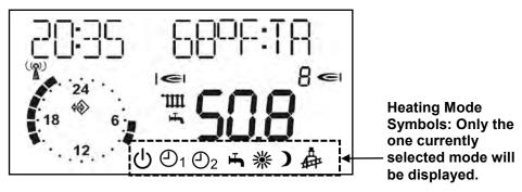
Figure 4-3: E8 HEATING Mode Display Features (NORMAL Mode)
