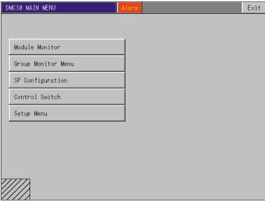
To display the "DMC10 MAIN MENU", press the lower left corner (the diagonally shaded areas in the above screen example) for at least 3 sec.
