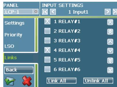
14. Once the links are complete, save the changes by selecting the 'Green Check' button in the lower left corner of the display.
