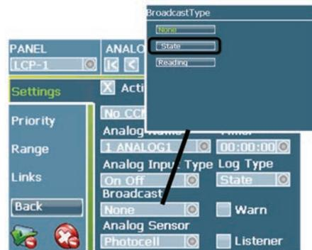
7. Touch the ‘Green Check’ button in the lower left corner of the screen to save the analog settings.
