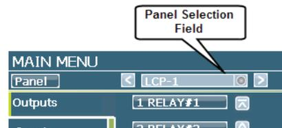
2. If the correct panel is not selected, select the 'Panel Selection' field at the top right of the display. The 'Current Selected Panel' display will show.
