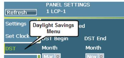
3. If your area observes Daylight Savings Time, make certain that the 'DST Enable' checkbox has an 'X' in it. If your area does not observe Daylight Savings Time, remove the 'X'.
