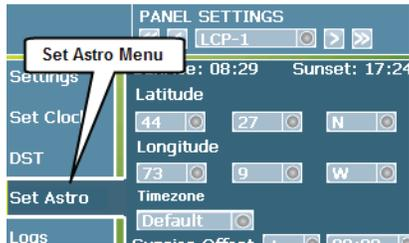
3. Touch the 'Latitude' entry boxes to activate the entry keypad. Use the 'Delete' button to delete the current entry before entering your location's latitude coordinates. Fields are in degrees and minutes format.
