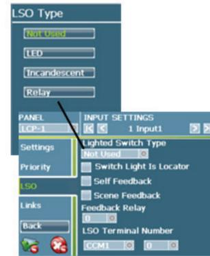
6. In the Greengate system, it is possible to choose from pilot light or locator light functions. For pilot light functions, leave the locator block unchecked. For locator light functions place a checkmark in the locator selection box.
