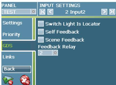
11. Use the 'Green Check' button in the lower left corner of the screen to save the input settings.
