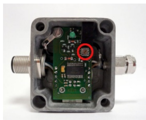
Fig. 6: CON. USB.WT Switch position
