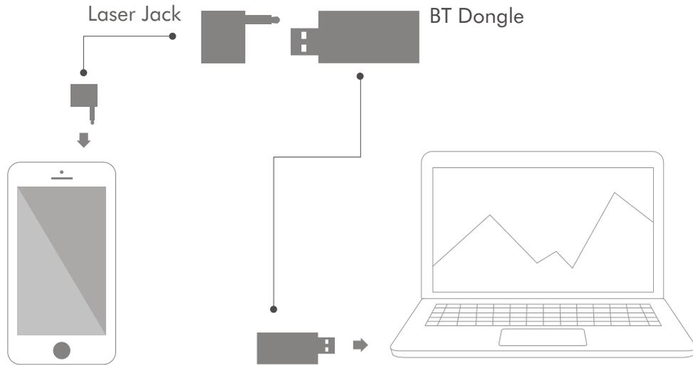
Plug in BT Dongle to target device's available USB port. Plug Laser Jack to Mobile device's Audio Jack.
