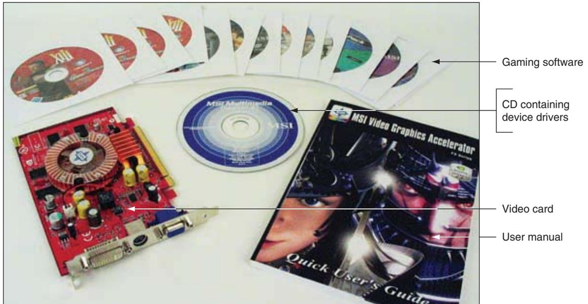
**Figure 2-13** A device such as this video card comes packaged with its device drivers stored on a CD; alternately, you can use device drivers built into the OS
