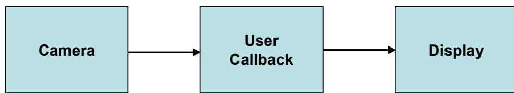
The API user can set data format passed to the callback function regardless of the image format streamed out by the camera by setting the argument of the ImCamOpen function.
