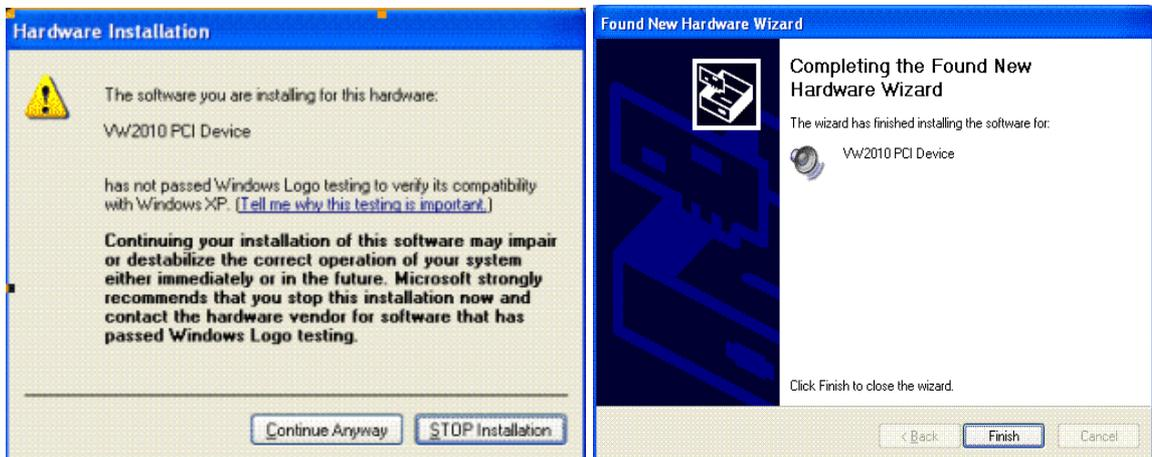
Installation of the other device driver "Phillips DVR" is similar as above. Alternatively, running the "**SetupDrivers**" program from the **Start->All Programs->Inventa->MPEGIO** program group after installing **MPEGIO** application software (See below) will have the same effect. Note the "**SetupDrivers**" program can also be used to re-install **MPEGIO** device drivers. Also note another installed program "**ResetDrivers**" can be used to reset the **MPEGIO** hardware if malfunction happens.
