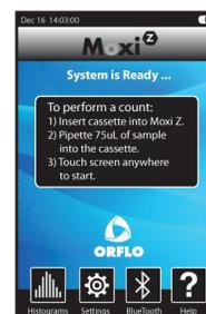
3. Press the tray down and insert a Cassette into the Moxi Z. The **Pipette 75 $\mu$ L Sample...** screen will be displayed.
