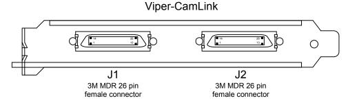
The hardware installation process is completed with the connection of a supported camera to the Viper-CamLink board. The camera will have one or two Camera Link MDR-26 connectors plus a connector for an external power supply. Connect the camera to the Viper-CamLink J1 connector with a Camera Link cable. If required, connect the second camera connector to Viper-CamLink J2. Refer to section "Connector and Switch Locations" on page 33.
