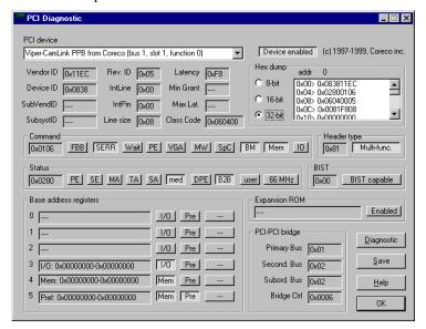
Click on the **Diagnostic** button to view an analysis of your PCI configuration. The **Information** message box contains the diagnostic report. If there is a problem, click on the **Save** button. A file named '**pcidiag.txt**' is created with a full dump of the PCI configuration registers. Email this file to the Coreco Imaging Technical Support group with a full description of your computer. For contact information see "Technical Support" on page 52.
