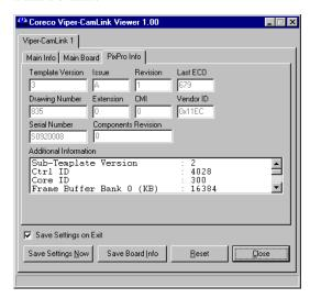
For Viper-CamLink boards with the optional Pixel Processor module installed, the **PixPro Info** tab displays information such as serial number and board revision of the Pixel Processor.
