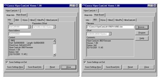
The **Main Board/Info** tab displays information relating to the Viper-CamLink onboard firmware. The scroll window named **Content** provides firmware details such as version, release date, etc.
