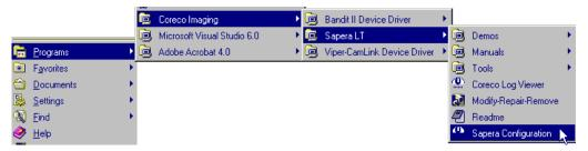
The Sapera configuration program (Start•Programs•Coreco Imaging•Sapera•Sapera Configuration) allows the user to see all available Sapera servers for the installed Sapera-compatible boards.
