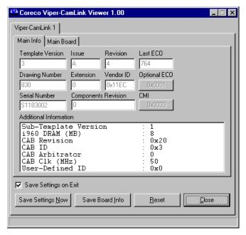
For each board, the **Main Info** tab displays information relating to the Viper-CamLink board issue, revision, and ECO (engineering change order) level, along with the board serial number and optional ECO or CMI (customer modification instruction) applied. The **Additional Information** window displays supplemental design data about the Viper-CamLink.
